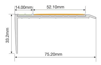
custom made photoluminescent pigment are embedded in thermoset polyester carriers to integrally bond the active ingredients into the aluminium following curing at high temperature. The photoluminescent area is also recessed into protective channels.
