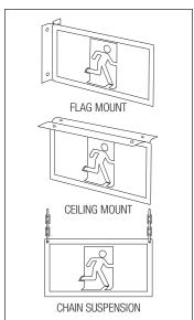
Ecoglo "Exit Right" S20 Signs are designed to clearly mark the direction of travel to the nearest exit. The signs will be clearly visible and readily understandable under all conditions of foreseeable use, including emergency conditions.
