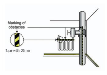
The UL-HZ2503 Hazard Tape is designed to ensure visibility of obstacles in escape routes for compliance with NFPA 101 Life Safety Code (NFPA 101) and International Fire Code (IFC). The Hazard Tape will be effective in all light conditions including failure of the main lighting.
