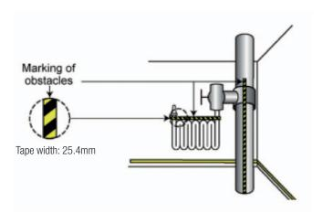
The UL-HZ2518 Hazard Tape is designed to ensure visibility of obstacles in escape routes for compliance with NFPA 101 Life Safety Code (NFPA 101) and International Fire Code (IFC). The Hazard Tape will be effective in all light conditions including failure of the main lighting.
