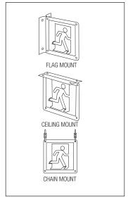
Ecoglo "Pictogram Uni" S20 Signs are designed to be used in and about buildings to identify escape routes for compliance with performance based building codes. The signs will be clearly visible and readily understandable under all conditions of foreseeable use, including emergency conditions.
