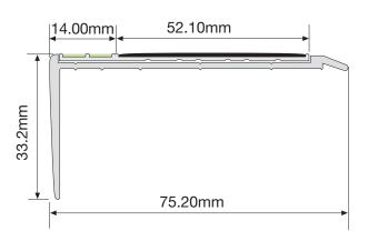
Ecoglo E14-075 Step Edge Contrast is adhesively fixed into the extrusion. The high visibility E14-075 is manufactured from extruded 60605T aluminium section. Silicon Carbide anti-slip materials and custom made photoluminescent pigment are embedded in thermoset polyester carriers to integrally bond the active ingredients into the aluminium following curing at high temperature. The photoluminescent area is also recessed into protective channels.
